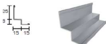
PROFILE "Double L" 25X15X8x15 L=3050 mm
