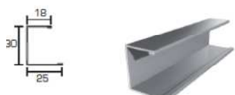
PROFILE "Double L" 25X15X8x15 L=3050 mm
