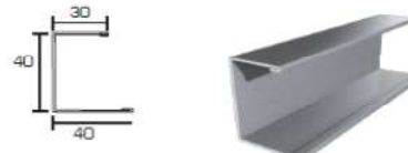
PROFILE "C" 30x40x40 L=3000mm
